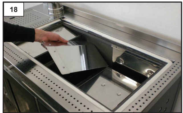
Remove the flue deflector located between the combustion chamber and the cooking oven (Figure 17 and 18).
