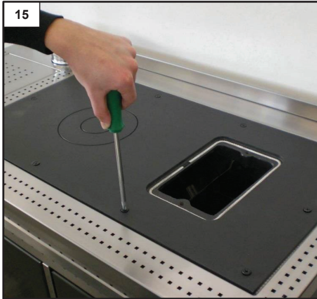
Remove the cooking plate by loosening the ten screws all around it after dismantling the upper cleaning outlet (Figure 15 and 16).
