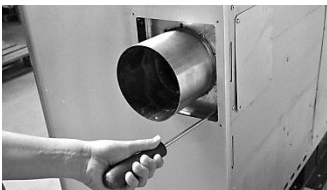
Install the sliding rosette by using bolts previously used to attach the inner protective lid
