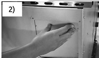
2) Remove the sheet beneath the lid by pressing onto the weakest juncture
