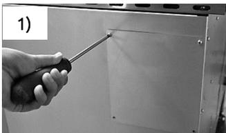
1) Remove the external protective lid with a screwdriver
