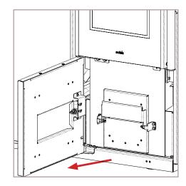
Open the ash pan using the handle, as in the figure below:
