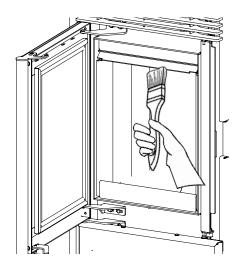
Vacuum the slide, the hatch and the surface hidden by the flame trap, paying attention not to knock the vacuum cleaner nozzle off the vermiculite.
