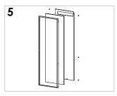
**5** Remove the majolica from the cladding kit, place it in the frame and close the group.
