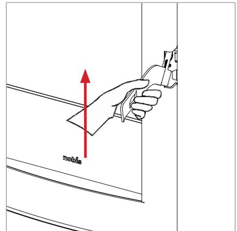
To extract the flame trap, lift it slightly as in the figure below:
