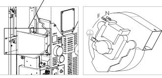
Make the electrical connection of the fan using the CANAL appendix, already present in the original wiring of the product. Live and Neutral can be inverted, unlike the earth connection (yellow / green colored cable) which must be connected to the earth of the fan.
