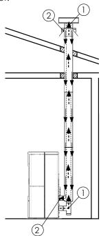
For coaxial installation or air sampling directly from the outside, it is recommended not to exceed 2.5 / 3 linear meters in order to ensure correct oxygen supply to combustion.
