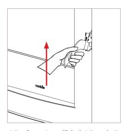
To extract the flame trap, lift it slightly as in the figure below:
