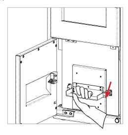
Remove the ash pan and empty it, as in the figure below:
