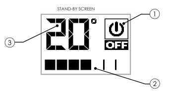
After 20 seconds of inactivity, the display on the handheld device blacks out and passes to "SLEEP" mode, maintaining the remote connection with the appliance. The display re-enables only by pressing the () key.
