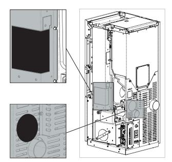
The installation of the ducting, without removing the pre-drilled hole blank, will result in NO heat being emitted from the ducting.
