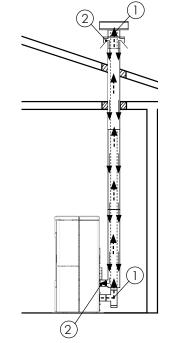
For coaxial installation or air sampling directly from the outside, it is recommended not to exceed 2.5 / 3 linear meters in order to ensure correct oxygen supply to combustion.
