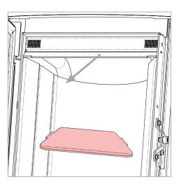
With a soft bristle brush, eliminate the combustion particulate, allowing it to fall in the slide beneath.
