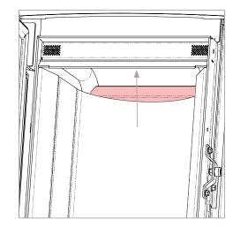
Remove it by bringing the lever towards you with slight movement downwards as in the figure below:
