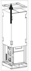
To remove the appliance from the pallet, you can remove the two screws placed under the pallet (13 hex key) to release the appliance from the wooden base.
