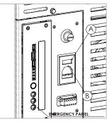
The "I/O" (A) switch in the figure above must be positioned on "I". In the event of a power failure, check the condition of the fuse placed under the switch (B) (4A fuse *EU configuration*). During periods of non-use, you are advised to disconnect the cable powering the appliance, and also the batteries from the handheld device.
