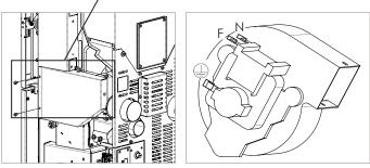
Make the electrical connection of the fan using the CANAL appendix, already present in the original wiring of the product. Live and Neutral can be inverted, unlike the earth connection (yellow / green colored cable) which must be connected to the earth of the fan.
