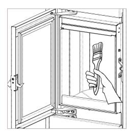
Vacuum the slide, the hatch and the surface hidden by the flame trap, paying attention not to knock the vacuum cleaner nozzle off the vermiculite.
