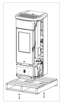
Position the equipment and proceed with its connection to the chimney flue. Find, using the 4 adjustment feet, the right level so that smoke discharge and the pipe are connected correctly.
