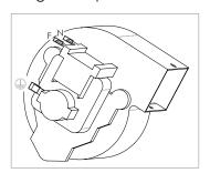
Live and Neutral can be inverted, unlike the earth connection (yellow / green colored cable) which must be connected to the earth of the fan.
