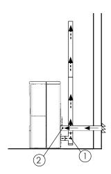
• smoke discharge (1) and oxidising air channelling (2) taking advantage of its coaxial discharge to expel the smoke and pick the air; therefore, installation is not necessary of a grate to recirculate the air inside the premises where the the product.
