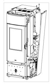
Remove the pre-drilled blank from the sheet metal with the assistance of a suitable tool (e.g. pry with screwdriver).
