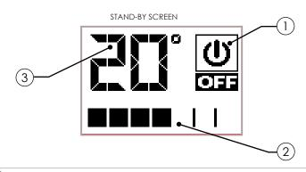
After 20 seconds of inactivity, the display on the handheld device blacks out and passes to "SLEEP" mode, maintaining the remote connection with the appliance. The display re-enables only by pressing the (1) key.
