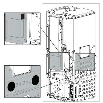
The installation of the ducting, without removing the pre-drilled hole blank, will result in NO heat being emitted from the ducting.
