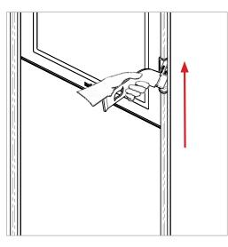
With a soft brush, eliminate the combustion particulate, letting it fall in the ash slide.
