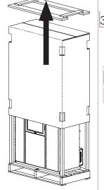
Toremove the appliance from the pallet, you can remove the two screws placed under the pallet (13 hex key) to release the appliance from the wooden base. Position the product and proceed with its connection to the
