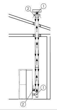
For coaxial installation or air sampling directly from the outside, it is recommended not to exceed 2.5/3 linear meters in order to ensure correct oxygen supply to combustion.
