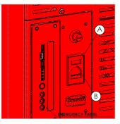
The "I/O" (A) switch in the figure above must be positioned on "I". In the event of a power failure, check the condition of the fuse placed under the switch (B) (4A fuse *EU configuration*). During periods of non-use, you are advised to disconnect the cable powering the appliance, and also the batteries from the handheld device.
