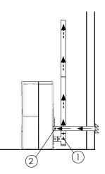
• smoke discharge (1) and oxidising air channelling (2) taking advantage of its coaxial discharge to expel the smoke and pick the air; therefore, installation is not necessary of a grate to recirculate the air inside the premises where the the product.
