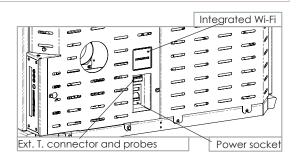
I It is compulsory for the system to be grounded and have a differential switch in compliance with legislation in force. Furthermore, ensure the socket is compatible with the type of plug on the power cable used.
