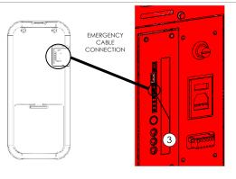
Before connection using the emergency cable, remove the batteries from the handheld device from the specific compartment. DANGER OF FIRE
