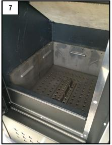
Now open the fire door to access and make the plumbing connections inside the combustion chamber (figure 6). Once the connections have been made, reverse the above procedure, carefully replacing all the parts previously removed, paying particular attention to repositioning the cast iron grate as shown in the photo above (figure 7) to prevent ash from compacting and falling into the ash drawer, which would reduce the flow of combustion air.
