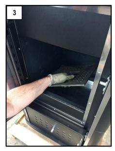
Remove the five cast iron partitions inside the combustion chamber (figure 1). Next, remove the cast iron grate (figures 2 and 3).
