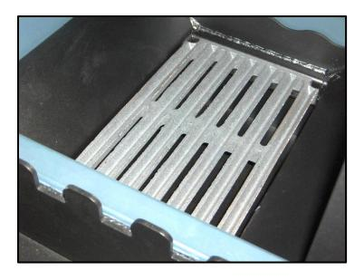
Replace the cast iron grille, taking care not to install it upside down, otherwise the ash will tend to compact in place without falling into the ash drawer.
