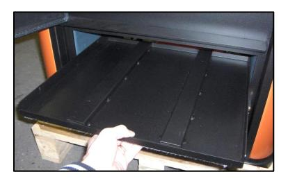
Pull out the ash drawer, then undo the four bolts securing it and remove the base.
