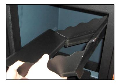
First remove the cast iron grille, then extract the grille mount.
