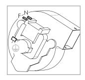
Remove the pre-drilled grid to allow the wiring to pass from the contact thermostat to the air fan (see wiring diagram at the end of the manual for further details).
