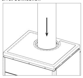
ATTENTION TO THE SECTION OF THE SMOKE DUCT WHICH MUST WIDHSTAND TEMPERATURES THAT CAN EASILY REACH 600°C.
