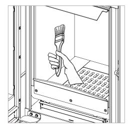
Vacuum the firewood support surface, taking care not to hit the vermiculite with the nozzle of the vacuum cleaner.
