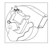
Remove the pre-drilled grid to allow the wiring to pass from the contact thermostat to the air fan (see wiring diagram at the end of the manual for further details).
