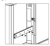
For models equipped with drawer, it is necessary to remove the drawer before installing the kit by acting on its rails with the 2.5 wrench (M4 screws).
