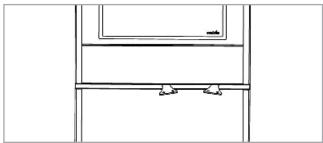
Combustion is efficient and "clean" when the flame looks pale yellow. If the flame tends towards red, or if you notice black smoke in the combustion chamber, turn the handle in the middle to slightly increase secondary air.
