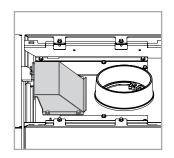
Lift the cast-iron top cover and fix the air conveyor with the size 8 key (M5 screws).
