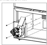
Following the holes (see arrows), fix the ventilation kit to the internal rear plate with a size 8 key (M5 screws).
