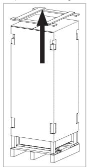
The body must always be moved in a vertical position using trolleys.
