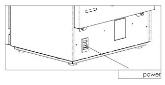
It is mandatory that the system is equipped with both earthing and differential switch, as per the laws in force. Also, make sure that the socket is compatible with the type of plug on the power cord used.
