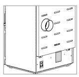
Remove the pre-drilled hole on the back of the product and, following the hole pattern (see arrows), fix the ducting kit to the internal rear plate with a size 8 spanner (M5 screws).
