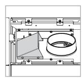
Lift the cast iron top and fix the air conveyor with the size-8 key (M5 screws).
