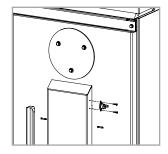
Remove the rear side with the size 8 key (M5 screws), take the contact thermostat from the kit box and connect it to the side of the air duct using a Phillips screwdriver.
