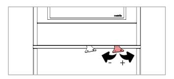
The central handle controls secondary air and is used to adjust combustion when the stove is running. Secondary air is fully open when the handle is turned to the right (+), while it decreases when the handle is moved to the left (-).
