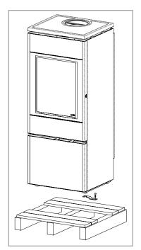
To remove the appliance from the pallet, unscrew the metal supports holding it, so as to release it from the wooden base.
