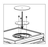
With the 3 M5 screws, fix the collar where the cap was previously removed and connect the horizontal section of the smoke duct;
