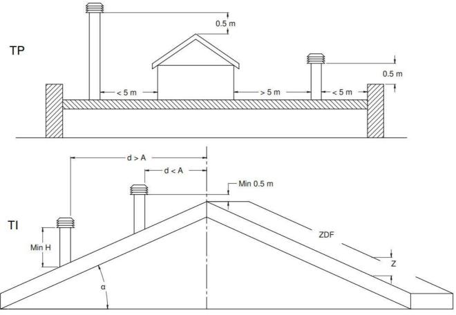
Key: TP - flat roof; TI - sloping roof; d - distance; ZDF - reflux zone
