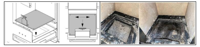
Vacuum the fire bed with an ash vacuum cleaner or remove the ash with a brush to ensure correct coupling. Suck up the ash that can get stuck in the front primary air slot or through the 3 front holes.
